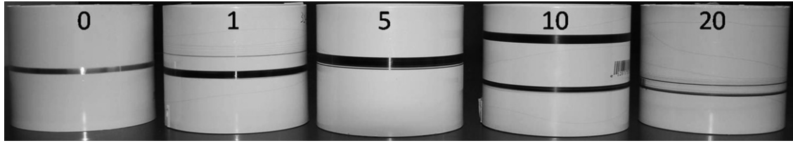
Fig. 1. Photograph of PEK and various PEK-g-FWNT fibers. The numbers on fiber spool represent the FWNT concentration.
